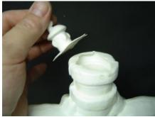
I used a knife to carve the mini blind rod so it fit snub in the square on the motor. You can see this on the left. I also cut off the knob that holds the head in place on the skeletons neck. I saved the knob for reconnection later.
