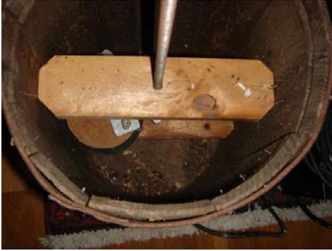
To start this project cut two pieces of 2 X 1 that are 9 7/8 inches long. This will keep the threaded rod centered in the barrel. The four corners on the pieces of wood you should cut off.
