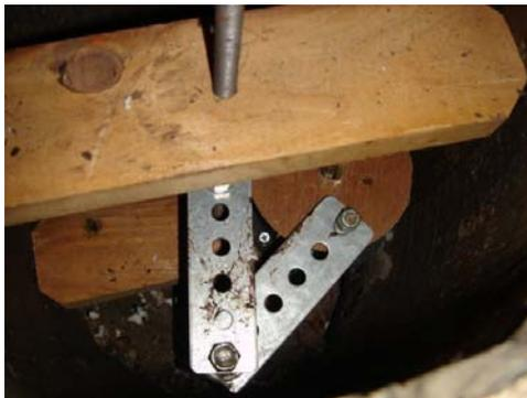
Place the motor on the piece of wood that you are using as a shelf. Move the motor as close as you can to the wall of the barrel with out any part of the motor touching the wall then screw the motor into the wood using some wood screws. Also go ahead and drill a hole in the back of the container for the plug to come out of.
