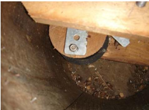
Take two pieces of steel flat bar that has the holes in it and cut two pieces that are 4 1/2 inches long. You should grind the corners of the flat bars to get rid of the sharpness.
