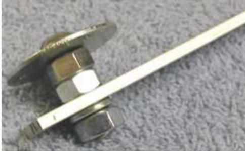
Mount the washer mechanism to the end of the arm with the 1/4" hole using a 1/4" lock washer and 1/4" nut.
