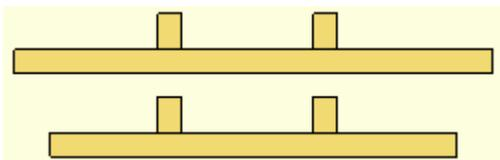
Next, we'll attach the 2" long pieces of 2x2's to the tops of the front and back 2x2's. They'll go about 6" each side of center (12" spacing) on each board. Drill pilot holes up through the front and back boards and into the 2" blocks. Attach with 2 1/2" wood screws.
