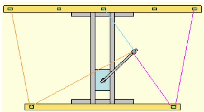
The drawing at left shows the routing of the three pieces of fishing line. After it passes through the front screw eyes, leave enough hanging for attachment of the skeletons as shown below.
