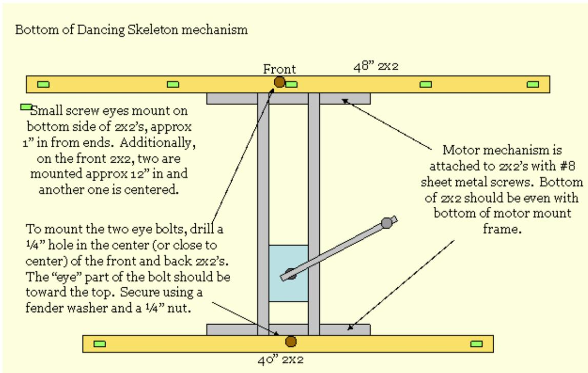
Attach the front and rear 2x2 boards to the motor mechanism as shown above.
