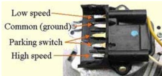
Before mounting the dancing skeleton rig to the ceiling, you'll need to wire up the motor. I recommend wiring it for low speed operation by attaching wires to the "low speed" and "common" terminals as shown at right. Note that part of the plastic housing has been cut away for easier access to the terminals. Soldering is the most reliable method of wire connection. For more info, see my [Wiper Motor Pages](#).
