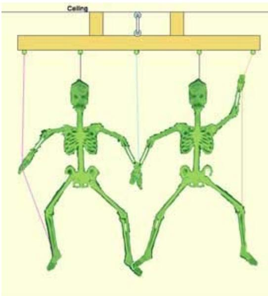
For mounting to the ceiling, you'll need to screw the large screw eyes into something solid in the ceiling, probably a ceiling joist. **Please be aware that just screwing them into drywall or plaster without solid backing will not work and you risk the high probability that the rig will fall and injure someone.**
