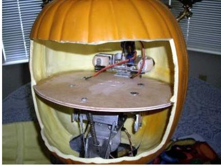
This project was turning out a bit front heavy, so it required a "counter balance" spring to take some load off the nod servo and linkage.
