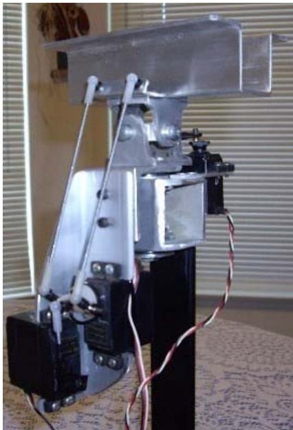
Then the "U" joint was fabricated using aluminum channel. The cross block is made from 3/8" thick stock. After drilling and tapping, bushings were used for smooth movement. Here you can also see how the tilt/nod servo bracket was mounted to the bottom of the "U" joint. The pan servo is mounted to the main bearing block and moves the universal joint.
