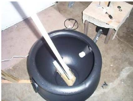
The stirpot wasn't hard to make. I used a bought cauldron, as large as I could find, and added an old rotisserie motor from a grill. It is attached to a piece of wood that is screwed to the bottom. I then added a piece of 3/4" dowl to a piece of aluminun stock connected to the motor and placed a 2' piece of PVC over that.. I plugged it in and it worked like a charm. You just have to remember to off set the motor a bit and make sure it doesn't have too large of a radius.
