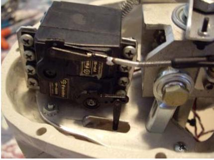
In this pic you can see the jaw servo at the bottom with linkage arm passing through the mounting plate. You can also see the pivot block mounted to the rod ends as well. Everything is mounted to an aluminum plate for strength and ease of installation.
