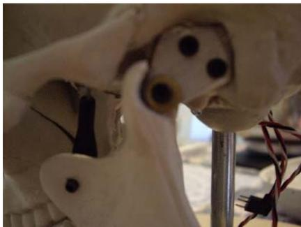
The first thing needed was a solid, smooth operating jaw hinge. After a little work with a Dremel tool I mounted a small piece of aluminum to the skull and used a 4/40 bolt through a nylon bushing into the jaw as the pivot. You can also see the rod attachment to the jaw in the pic below.
