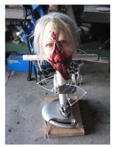
Now until you see it for yourself, the motion is hard to describe. The best way we can put it is like how the Earth revolves around the sun. The motor and PVC will act like the Earth. Just as the Earth spins while going around the Sun, so will the PVC that is attached to the motor. Now as long you don't want a tornado zombie spinning in the ground, you will have to not only control the path around the sun, but eliminate the spinning.
