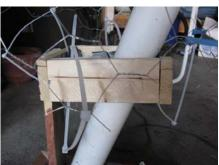
We built a frame to control the motion of the zombie. This way the motor does not go too far in one decoration and not be able to pull itself back up. We also used tie straps to control the spinning so that the zombie will only look in one direction.
