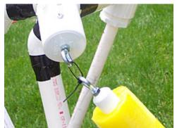
The 45-degree elbow fittings each connect to an end cap fitting. An O-ring bolt is mounted thru a hole drilled in the center of the end cap.
