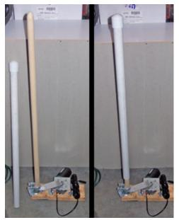
The stirring stick is made of two pieces. A 3/4" x 3' wooden dowel is attached directly to the motor arm.
