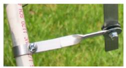
The other end of the lower arm is connected with a short bolt and lock nut with washers on both sides and in between. This connection must be loose enough to allow ease of movement.
