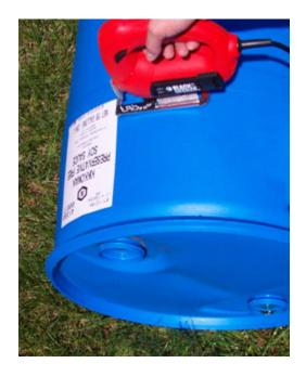
I cut the top of the drum off with a jigsaw just above the top "strap". Make a starter hole for the jigsaw blade with an appropriately sized drill bit.
