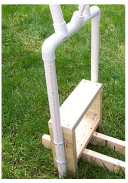
The PVC legs are attached to 90 degree elbow fittings on each side and three T-type fittings in between.
