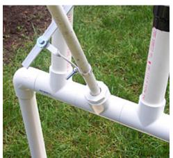
The lower arm is made of lightweight aluminum stock that was bent around the 1/2" PVC and attached with a screw and nut. In this picture, you can see how the 1/2" pipe is going thru the 3/4" reducer into the T-connector. The 1/2" pipe must be loose here. The reducer just acts as a guide. The end cap (which is hidden from view) provides the spin point at the bottom.
