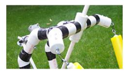
The "shoulders" are formed from two T-fittings, two 45 degree elbow fittings and one 4-way junction. The 4-way has a 3/4" reducer on the section pointing down. The reducer acts as a guide for the 1/2" PVC "neck".
