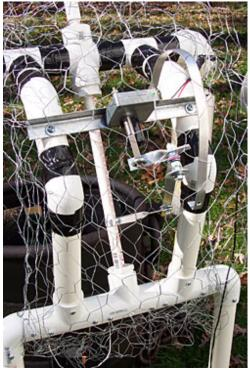
There has to be enough clearance in the wire form to prevent the turning motor crank from catching. I made sure there was enough room by attaching a bent piece of aluminum stock to the motor mount. The wire form could not be pushed past the aluminum.
