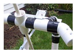
The 1/2" PVC "neck" is guided thru the 4-way connector with another 3/4" reducer. Once again, the reducer just acts as a guide. The 1/2" pipe must be free to turn at this point. Both of the reducers are dry fitted into the connectors so they can be removed if necessary.
