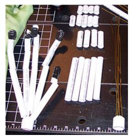
The 1/4" diameter of the pipe was about the size of the fingers in the latex hand. Again using the latex hand as a guide, I cut pieces of the pipe to match the approximate length of each of section of a finger between the joints. There were four pieces of pipe for each finger and two sections for each thumb.
