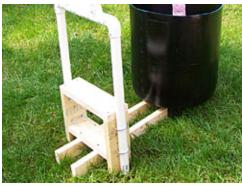
The witch frame is built on a base made of 2"x4" and 2"x6" lumber screwed together for easy disassembly.
