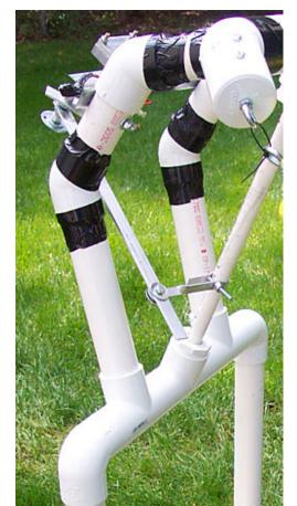
Two 45 degree fittings and three sections of PVC pipe form the "sides". I used black duct tape to secure some of the joints. This made it easy to adjust the angles. The "sides" are also used to mount the motor that will turn the witch's head.
