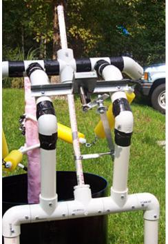
The motor that turns the "neck" is a 6 RPM 12vDC gear motor that I purchased from www.allelectronics.com, however they do not seem to have that motor that now.
