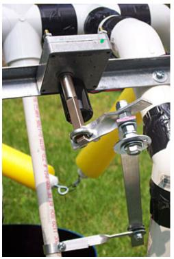
A short crank arm made of aluminum stock is attached to the motor.
