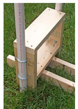
Four U-bolts are attached to the 2x6 uprights to hold the PVC frame. The frame is made out of schedule 40, 1.5" PVC pipe and fittings. Two 33" sections of 1.5" PVC pipe form the "legs" of the witch.
