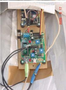
Tied to the output of the uMP3 is a Cowlacious Design's Scary Terry servo driver card that takes the sound generated by the uMP3 and controls a servo in the Witches' skull/head, as well as a pair of eerie green LEDs mounted in the eye sockets.
