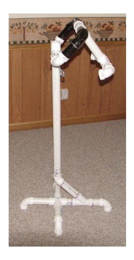
I don't have any real measurements so you will have to sort of play it by ear. You will notice that the one leg is longer and that was the back leg to help support the body. Since there would be a rocking motion and the arms were going to be pushed back I decided to add this for support.
