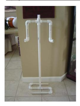
I started with a simple 1" PVC frame. I had to use a heat gun to get the angle of the PVC on the arms right since they don't carry a fitting that bends in that degree at any stores close by.
