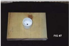
FIG. #7 Screw a 1 1/2" PVC End Cap to a wooden base.
