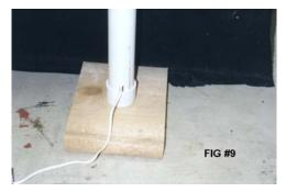
FIG. #9 Feed the power cord through the notch on the bottom of the post and secure the post in the PVC End Cap on the wooden base.
