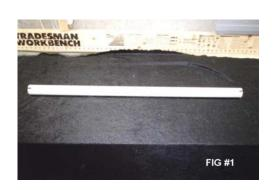
FIG. #1 Cut a 10' section of 1 1/2" PVC into 1/3's, which will give you 3'4" posts. Make 2" x 1/4" notches at the top and bottom. Make sure you cut the notches on the same side of the PVC section.
