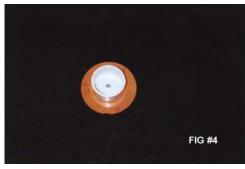
FIG. #4 Secure the PVC End Cap to the plastic base with a small nut and bolt. This shows the bottom of the plastic base and inside the End Cap.
