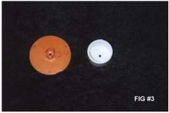
FIG. #3 Drill a small hole in the center of the plastic base underneath where the light bulb fixture seats. Drill another hole in the center of a 1 1/2" PVC End Cap.
