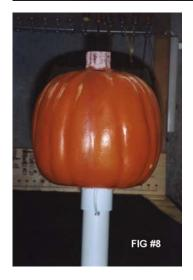
FIG. #8 Feed the power cord from the Pumpkin down into the PVC post and through the notch on the rear of the post. Attach the Pumpkin to the top of the post with the PVC End Cap.
