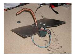
The next step is to make the "shaft". In this case what we really need is for the shaft to stick up an inch or two and then turn to the side. The end result will be like a big slow mixer with the shaft hitting the chains and making the whole thing move. I couldn't really find anything appropriate so, since this doesn't have to withstand a lot of torque, I just took some copper tubing and crimped it down so it would fit the motor shaft.
