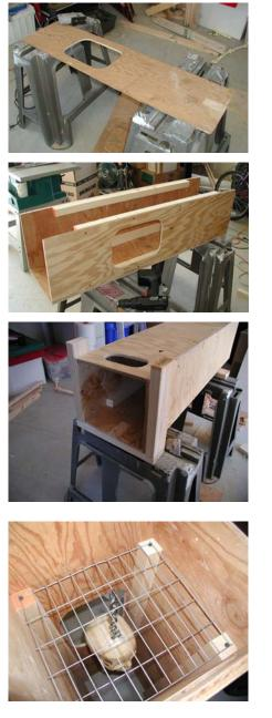
Construction of the box was fairly simple, 4 panels 1 foot by 4 feet are cut from plywood. The front piece has a hole cut in it that is 18 inches high by 10" wide (the maximum width permitted by the side braces.) The back piece has a hole for access and airflow cut in at the top and bottom, the exact position doesn't matter.
