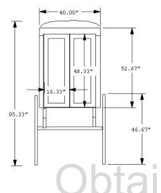
Here are the general dimensions for the hearse size, yes it really is that big. I made it in two parts the back part is for the coffin and the front seat section was added to it after it was made.
