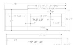
I started out making the coffin to the size on the drawings out of oak plywood. I had just enough scrap walnut to do the cross on the top with. I did the edges of the plywood with 1 1/4 inch wide solid oak stock with no inlay, this cut down the cost.
