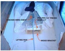
I dressed him in an old shirt and tie and attached a 1 inch wide piece of aluminum stock to the frame and down to the sliding block on the ram. At the end of the ram I made a switch out of two pieces of wire that activated the scream from the digital chip recorder from Radio Shack. The speakers are under the hearse and are cheap powered computer speakers from big lots.
