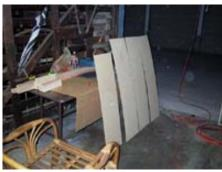
The Hardboard needs to be cut into: 3 - 4' x 1' 1 - 3' 6" x 1'
