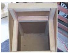
We cut an inside piece so the money didn't fall all the way down. Of course since I'm lame and my measurements never come out right, we had to put a few small pieces against the sides to make it a nice tight seal so coins don't go through. This doesn't matter because nobody's going to see inside
