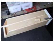
Now the corner and ground molding is cut. I had to cut the ground molding using a Miter Box to get the 45° angles.
