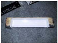
Again, I skip a few steps. This is the box that fits on top for the sign. It's just two small evenly cut 1½" pieces with a 1½" x 1' and 2½" hard board attached to the top and back respectively.
