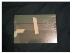
Here's the piece of plexiglass. It comes with a film on it so it doesn't get scratched. I cut the piece out by scoring it with a mat knife about 987497394758 times. Finally, I was able to bend it down the score and it snapped cleanly apart.
