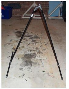
Here's the base. From the bottom up: four 12" pieces into T connectors. Extended T connectors screwed onto 36" legs. Left leg is then screwed into a 45 degree elbow which is then screwed onto a nipple and then a T. Right leg assembly is screwed into the same T connector. This piece takes a little coaxing (a lot of coaxing), but is well worth the effort. **This joint must be tightened as securely as possible.**
