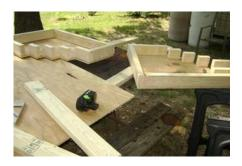
I cut out the sides, front and bottom pieces. I cut pieces of a stud to frame the inside and top of the carriage.
