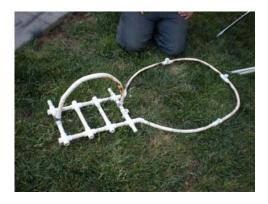
This is the basic frame of the spider. The rounded parts of PVC that you see were bent using a propane torch.
