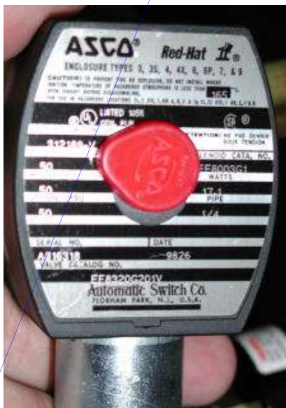
ASCO "Red-Hat" EF8003G1 (only rated for 50 PSI)
