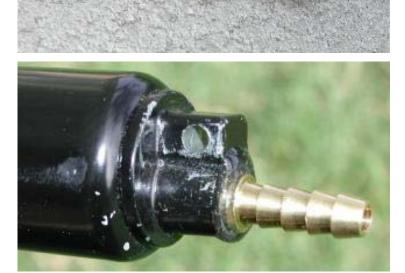
pour the epoxy between the barb and the inner wall of the hole.
