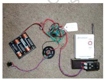
The <u>Radio Shack</u> recordable sound board is in the center. The <u>trigger relay</u> is lower right with the <u>X-10</u> module just above it. The wire from the sound board terminates in a 1/8" socket that connects to the <u>amplified</u> <u>speakers</u>.
