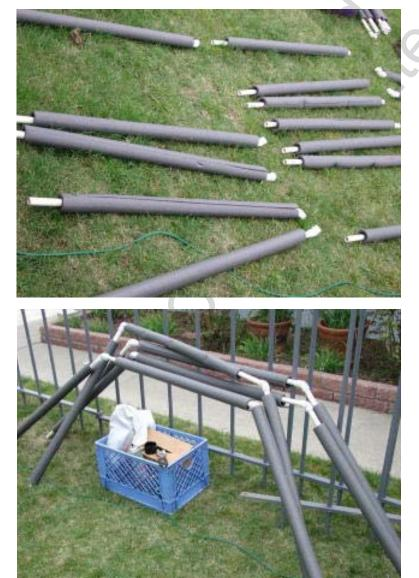
The leg pieces are sorted out. Each one is marked with the leg (letter) and joint (number).
