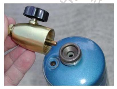
The center hold contains a check-valve that will only dispense propane when a properly designed appliance is screwed on.
