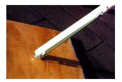
Six of the spider's feet touch the roof. Those legs don't need to be terribly strong, because they are supported at both ends. This is a foot pad, which anchors the far end of the legs.
