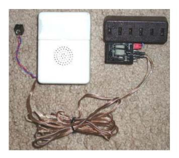
The canned scream is the big white box. The trigger relay is upper right. It is usually plugged into an X-10 module. The blue and red wires on the left from the sound box terminates in a 1/8" socket that connects to the amplified speakers.
