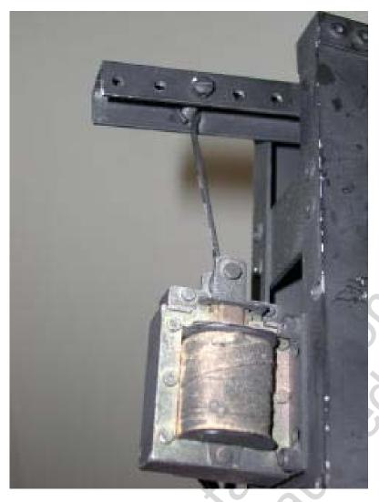
Parts are not critical, except that you get them to fit together. The solenoid is a 110 VAC pull model from the electronics junkbox. Leverage is used to give it strength, so it need not be particularly strong. Try the usual surplus stores: Jameco, <u>Hosfelt</u>, <u>MPJ</u>, <u>All</u>, <u>Goldmine</u>, <u>Herbach</u>.
