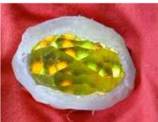
The spider was given a pair of eyes, made from faceted plastic "gems". Behind each gem was a pile of self-flashing LEDs, some yellow, some green. When activated, the LEDs twinkled, casting light through various facets.
