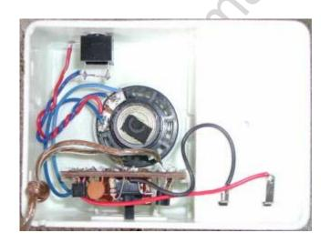
The final step is to drill a hole in the case and mount the socket. In operation, the <u>amplified speakers</u> plug in here.
