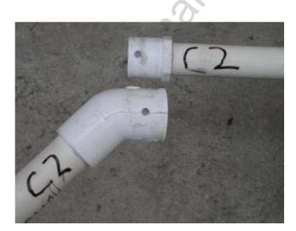
All of the leg sections are either glued or pinned.
