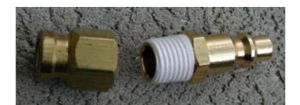
Put the rest of the parts together, using teflon tape on the joints.
