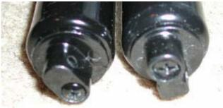
Find the air adjustment valve. It should be on the end of the cylinder body. It just looks like a screw. If you're lucky, it will be indicated by markings for "+" and "-" or "faster" and "slower". Most are unmarked.
