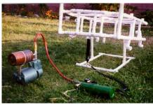
The spider is animated, because the only thing more terrifying than a giant spider is a giant spider lunging at you! The body is made to rock back and forth on a central pivot. Up front is an air cylinder that provides the motion. Although there is only one air cylinder in the spider, the rocking of the body causes all of the legs to move. When the spider lunges down at the victims, the front legs wave up and down.
