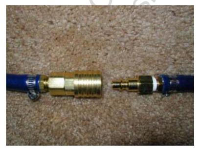
We like to give our components a common, standard connection. This allows us to move them around as required and replace tired units with spares. The snap-on air connectors are a key to this. Our compressor and all of our hoses and manifolds use these same quick connectors. Any time we want, we can add 50 feet of hose, a manifold, or another HAM - just by snapping it into place.
