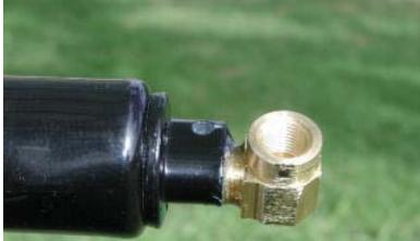
Tap the hole all the way through (inner and outer) with a 1/8" NPT tap.
