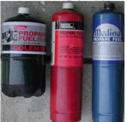
Here is an assortment of old propane cylinders. We use the little tanks, intended to power camping lanterns, soldering torches, and camp stoves. Technically, these tanks can be refilled, but it is illegal to transport them after refilling. Effectively, empty tanks are worthless.
