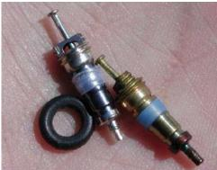
Both valves have removable spring "cores". Just unscrew them and they fall out. The valves cores themselves are similar to those used in automobile tires, and they unscrew the same way.
