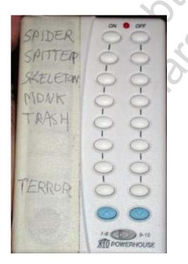
We used this PalmPad in 2001, with a masking tape label for each effect.
