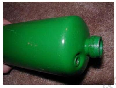
Construction is simple: get empty propane tank; make sure it's empty; unscrew and remove the two valves; wash out with soap and water; drill and tap for 1/4-inch NPT; clean; paint; replace the pressure relief valve.
