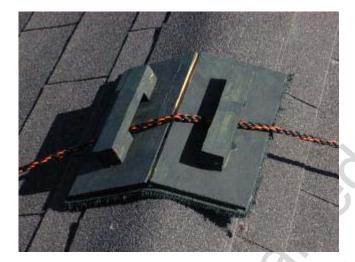
A PAIR of pads like these protect the roof against abrasion from the safety rope that keeps the spider from sliding down the roof.
