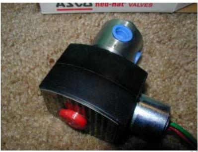
Each HAM has an electrically-controlled (solenoid) valve. It permits us to remotely cause air to flow from the storage tank to the prop. When we turn the valve back off, the air in the prop is expelled through the exhaust port.
