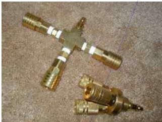
Both of the units shown here work the same way: they accept air through a male quick-connect; they dispense air through three female quick-connects. Note that the female quick connectors contain built-in valves so that air is not released through unused connectors.
