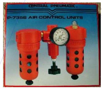
This unit from <u>Harbor Freight Tools</u> performs filtration, regulation, and lubrication.
