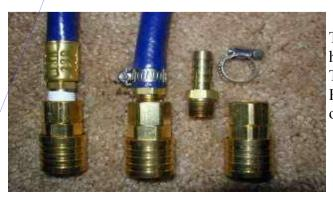
The connection in the middle was added to the cut end of a hose. First, a barbed connector was shoved into the end. Then a hose-clamp added to secure the barbed connector. Finally, the quick connect was threaded on the exposed end of the barbed connector.
