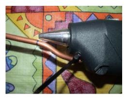
You want to bend the pipe so that it is parallel to the tip of the gun. You will want to play with this later though to get a good blowing result. Cut the pipe off flush with the end at a slight up angle to the tip.
