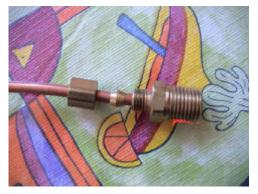
This fitting was a bit harder to find but it was a good find. It adapts the 3/16" copper pipe to a 1/4" air fitting using compression. You slide the top and the little ring over the pipe. Stick the pipe in the fitting and screw it on tight. Easy peasy!
