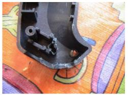
Here you can see how I had to drill out one of the screw posts to make room for the fitting. I will use that hole for a zip tie later.
