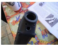
Drill a hole large enough for your 3/16 pipe to pass though the front of the gun. You want to drill the hole dead center on the flat section just below the nipple (see photo). I added a tie wrap as per the instructions from Brent Ross but I'm not sure if you really need to. If you choose to you want to drill 2 small holes just above and on either side of the larger one.
