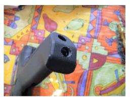
Now drill a larger hole at the bottom of the gun similar to the hole for the power cord. This will take some time to do as you will find that depending on what fitting you are using and what size of pipe you will have to remove some of the supports and plastic in the handle. I accidentally removed too much and have to use 2 zip ties to hole the handle tightly closed but it doesn't affect the function of the gun.
