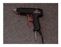
This is the completed gun. It's almost like they made that flat spot on the bottom so that I could put an air fitting there.
