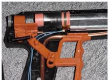
The heater wires originally ran where the copper tube is. In Several places I had to make the openings larger by melting with a soldering iron.
