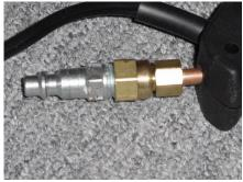
The air comes in through a common airline disconnect screwed into a brass female pipe thread to compression fitting. the screw hole in the handle above the airline is one of the screws I wasn't able to put back in. You can see the handle spreading slightly. Still, the handle is very rigid and it doesn't seem to affect it.
