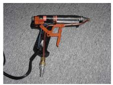
Here is the route the copper airline takes through the handle. I had to eliminate 3 screws to route the airline through. It doesn't seem to affect the strength as the shell is very strong. It could be glued together as there is really no reason to take it apart once complete.
