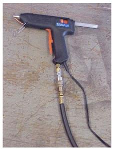
Ready to shoot. This thing can really suck down a glue stick. I don't have a valve on the gun. I adjust the air at the regulator that feeds this hose and just disconnect it when I'm done.
