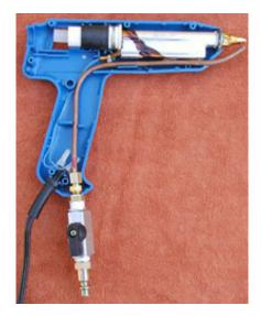
Install tubing assembly into gun as shown left. Note that your tubing will be longer at the front of the gun than the picture shows.
