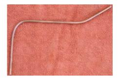
You'll need to bend the copper tube into the shape shown left. Copper tubing is easy to bend, it's important not to do too tight of a bend or bend it too quickly as it might kink the tube which cannot be undone.
