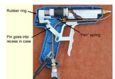
Reinstall trigger mechanism. Glue feed and trigger fit into slots in the case. Pin on arm that connects trigger and feed goes into recess in case.
