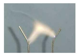
The basic construction and principle of a Jacobs ladder is that a metal vee is formed from two bits of wire and a high voltage is applied across them. The electricity arcs across at the bottom of the vee where the electrodes are closest together. The air that
