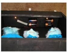
I decided to light the ghosts from above, so I bolted a couple battery holders inside the box at the top. I also mounted a couple flashlight bulb sockets to the light bezel. You will probably want to experiment with the number of batteries and light bulbs under the actual lighting conditions you will use. If the lights aren't bright enough, you won't see the ghosts. If they're too bright, the effect looks hokey.
