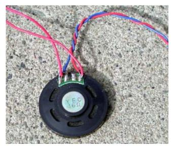
This is the speaker that provides the output for the Radio Shack sound board. The original pair of red wires run off to the upper left. All you have to do to get the sound from the board is to tap into these two wires.
