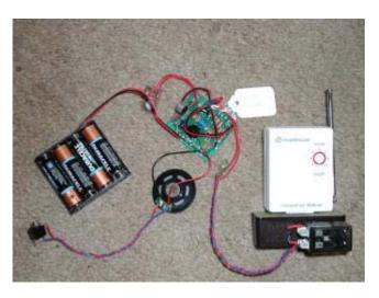
The <u>Radio Shack</u> recordable sound board is in the center. The <u>trigger relay</u> is lower right with the <u>X-10</u> module just above it. The wire from the sound board terminates in a 1/8" socket that connects to the <u>amplified speakers</u>.
