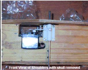
Note nosegear mount and head rotation linkage
