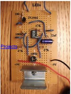
PARTS LIST: 1458 Dual Op-Amp, 22uf capacitor, 3 - 47,000 ohm resistors, 100,000 ohm resistor, 100 ohm resistor, 100,000 ohm potentiometer, 2N3904 transistor, 2 - LEDs.
