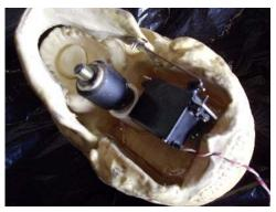
After removing the sound box a nice flat area was left to which a piece of thin ply was glued in using RTV adheasive. A perfect place to mount a servo and a way to mount the skull to a bracket.
