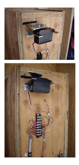
Door servo mounted to back. A larger servo arm was made to accommodate the longer throw necessary. This is a large servo made for really big model airplanes. (1/4 scale)
