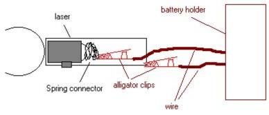
Since the alligator clip has the rubber protector around it I don't have to worry about it grounding against the case of the laser. Then a cheap battery holder from Radio Shack was attached to the wires and I have an easy-to-replace set of standard AA batteries for my Laser Eyes.
