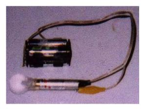
When installing the lasers into the skull I disconnect the clip on the body and slide the whole thing in, then re-connect it. The top of the skull hides all the batteries and wires!
