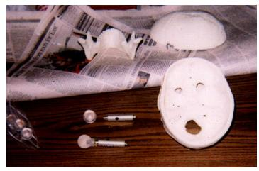
It may be difficult to see in the picture at left but the bottom laser pointer shows the complete effect, you can see a frosted ball glued (I used good old hot-glue) to the end of the pointer. Above it you can see a ball and a pointer and to the left is my bag of parts.
