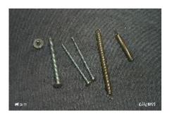
The springs are from my junk drawer so I do not have exact numbers on them, but they are 2.25 inches long in the compressed state, and 0.175 inches in diameter and are made from 0.020 inch spring wire. I needed a long one and a short one, so I just cut one in half and bent a few turns down to make a new end loop
