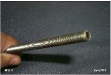
Then insert the spring assembly by screwing in both spring ends and slip the middle screw into the brass tube. If the head still tilts a bit too far forward when you hold it by the neck shaft, you may need to stretch the back spring a bit to make it longer. Remember to test the balance with the cap on, since the balance will be different with it in place.
