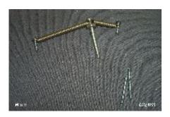
Assemble the springs and screws as shown. Do not tighten the nut against the springs. It is used to adjust the tension and moment arm of the neck shaft.
