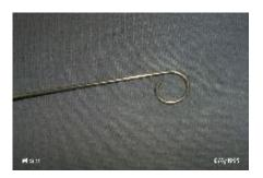
I started by bending a loop in the end of the wire. This gives the wire a bit of spring and gives a way to adjust the length of the pin if need be (by making the loop larger or smaller).
