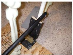
Step 6: With that same drill bit, drill two holes in the 3/4" PVC at 7" and 10 1/2" from the bottom of the PVC.
