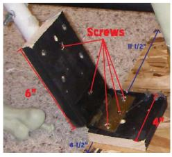
Step 1: I placed the 4" 3/4" piece of wood on one edge of the plywood base.
