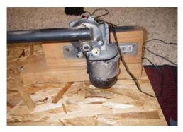
Step 2: Mount the motor to one of the 2X4's. There won't be a need to replace the crank arm for this prop.
