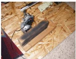
Step 3: Place the 2X4 not attached to the wiper motor to the plywood base. I placed mine about 16 1/2" from one side, adn about 4" from the other, as in the picture.
