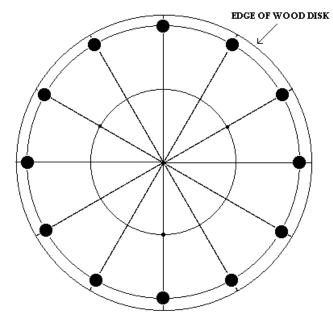
This will secure the disks to each other. Now drill twelve 31/64 inch holes at these locations, all the way through both disks.
