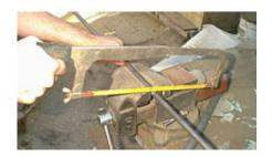
Using a hacksaw, cut off excess rod at the bottom and smooth with file.
