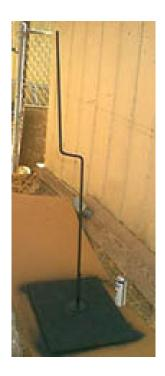
Clean the Steel Rod with soap and water to remove any oils that may prevent paint from sticking, then dry thoroughly. Spray paint the metal rod with flat black spray paint.
