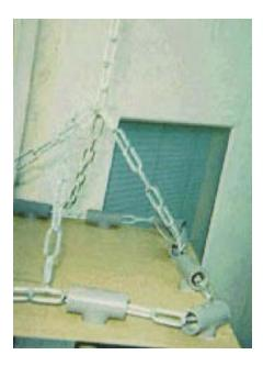
For the top I really wanted a chain. So I came up with the idea of using pipe T's and running a small chain through them. The chain was the cheapie \$.50/foot at OSH. Then I simply press-fit the pipes into the T's so I can remove them after Halloween and it will all collapse. You can see a close-up of the chain going through the T's to the left. To link the chain I just wired 2 links together, same with the 4 pieces that go up to the hook.
