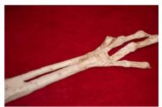
Eyeball the shape of the long shaft and grind out the ¼ "hole in the crank to match, so as to keep it in that 180 degree opposite position when mounted (about ¼ "from end of shaft).
