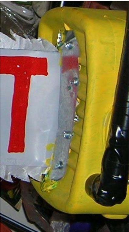
16. To make it more stable, I cut out two pieces of scrap metal, drilled holes in it, and screwed a plate into each side of the blade to prevent it from wobbling or falling out.
