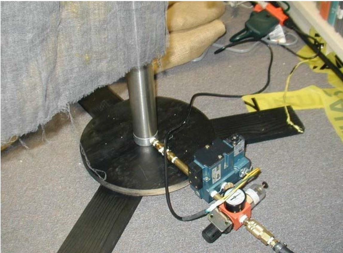
4 way solenoid valve used to trigger air cylinder
