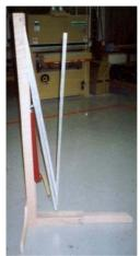
As soon as I tested the mechanism I learned that when the air cylinder fully deploys, it tilts out forward slightly, putting a bind on the cylinder sliding back down into the body of the pump. To counter this I used a hose clamp around the top of the pump's cap to hold one end of a small chain that limited the pump to perfectly aligned to the ram. No binding has occurred since.
