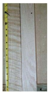
The placement of the 3/16" hole drilled for the pin is at 13 3/8" off the floor and 7/16" from the front edge of the frame. Drill in about 3/8" to 1/2" deep. Make sure your holes are exactly the same on both sides of the frame so the line up and leave the cylinder mounted square to the frame.
