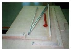
Here is our first look at the items making up the entire frame and mechanism together. We attached the lower points of the scissor sections to each other using 1/4" x 1 1/2" hex bolts. Cut your lower square tube down to 47" long and now drill a 1/4" hole in the bottom side. Drill the same hole in each of your other two sections as well. Remember to put these on center and 3/8" from the ends.
