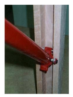
Once you have all your holes drilled and then attach the final side to your framework with 1 1/4" drywall screws and the 5/16" carriage bolts, your air cylinder should be "floating" between the two sides.
