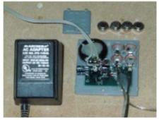
It's time for Regan to speak up. I didn't have a digital voice recorder handy for her voice, so I picked up a 10 second talking picture frame from Radio Shack. Hacking into it I ran one wire to the hot lead under the button that you push inside the photo frame to make it play back, and another lead to the opposite side of the panel the IC board it attached to for the ground.
