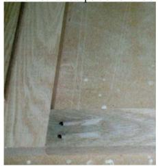
The l-shaped sides for both sides of your framework will be assembled as shown above using the pocket bore jig. Use a yellow wood worker's glue in the joint and be sure your cuts are square. Hold your two pieces of wood down FLAT to your work bench so your joint is flat and square. Be sure the screws pull up tight. Here are both sides and the center piece that will attach them to each other.
