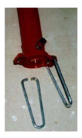
Now we turn to the air ram. We will need to mount the base somehow to the frame, so the way I chose is to use a section of one of the feet that is on the bottom. You can cut this to 2 3/8" or even 2 1/2". This "pin" will slide through the two holes that the foot used to clamp into and into holes drilled in to each side of the framework.
