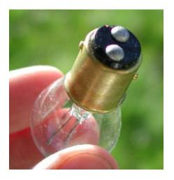
The bayonet socket is spring-loaded. You push the lamp down, then twist slightly to engage the nubs in the hook of the J-shaped slot. When you release the lamp, spring pressure pushes the lamp nubs up into the hook.
