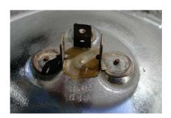
This is a headlight from my Mitsubishi Montero. A molded plastic connector pushes onto the blades to make contact.
