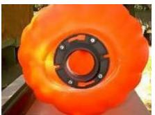
Place the closet flange over the large hole you cut in the bottom of the plastic pumpkin and line up the four bolt holes in the flange with the four holes you drilled in the bottom of the pumpkin. Push the bolts through the closet flange holes and the holes in the bottom of the plastic pumpkin. Now, reach in through the large hole and place a washer over each bolt, then put a nut on each bolt and tighten snugly with a wrench. Do not over tighten or you might break the plastic.
