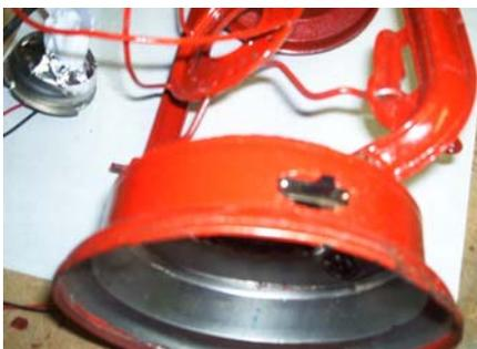
Drill a couple of holes in the side and trim out using some tin snips.
