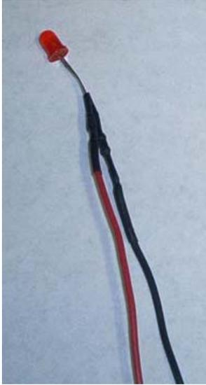
Cut the wires back on the resistor to about a 1/4". Solder the resistor wire (it doesn't matter which way it is facing) to the short wire of the LED. Then solder the other end of the resistor to the BLACK wire. Solder the RED wire to the longer wire on the LED. Place the Heat Shrink Tubing over the connections and lightly run your soldering iron over it to shrink.
