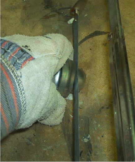
Cut off the top part of the wick assembly with a hack-saw. Use gloves for hand protection.
