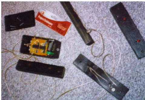
I assembled the all the electronics on a perfboard shown here screwed into the project box. Here's a view of that. Note the LED eye wood blocks shown to the right.
