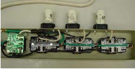
9. This is what you should have when you're done. Inspect the wiring to make sure that all connections are tight and that the soldered junction is insulated. Replace the cover on the strip.
