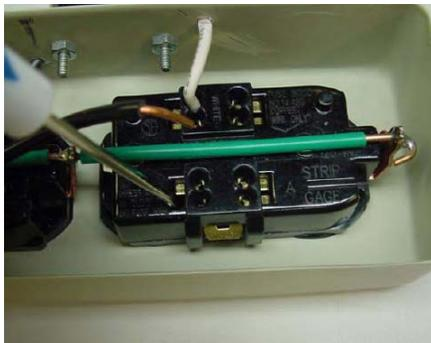
3. Open the back of the strip to expose the sockets. Using a small screwdriver press on the tabs to release the white wires. The picture shows a black wire, but you get the idea. The white wire in this pic is actually the wire from the starter socket.
