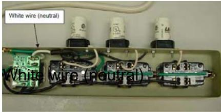
4. The white wire called out in this pic is the line that goes into the first socket. Pull it out of the outlet tab but leave it connected to the surge protector board.
