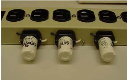
5. Drill some holes in the side of the strip housing where you want the sockets to be attached. You'll need two holes to mount the socket and holes for the wires to go through. You can see the ends of the screws in the pics in Step 3 and 6.
