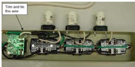
7. Repeat this process for the next two sockets. When all three are installed pull the three black starter socket wires along the inside of the strip as shown below. Trim and tin the white socket wires and insert them into the power outlets. Trim the white power
