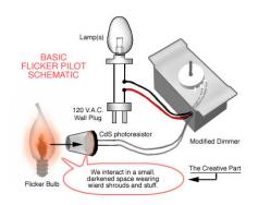
Once you have the modified dimmer completed, wire your test system up as shown at right. The CdS cell and flicker bulb should have a darkened space all to themselves. Since no two flicker bulbs behave the same way, every system will be unique, and will require experimentation to perfect.
