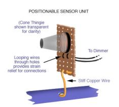
Since the necessity of occasional adjustments must be expected, mount the cell assembly so that it can be repositioned easily. One helpful suggestion is to mount the cell to a small piece of perforated circuit board at the time of wiring. You can then use an empty section of the board to accept a piece of stiff copper wire, as shown at left. The wire can then be screw-mounted to the box.
