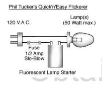
Can it get any simpler than the FlickerPilot? You bet! Phil Tucker sent us his favorite method, and it's about as simple (and clever) as can be. The circuit at right tells the tale. Using a fluorescent starter module (Home Depot), this gadget can handle up to 50 Watts of lights. I can hardly do better than this diagram in explaining it. This requires no elaborate enclosure. All
