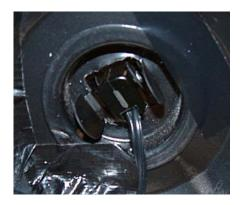
Christmas candle if you ask me) If you get the "standard" sized bulbs you can hack any old lamp you have lying around the house and use its socket & switch. I prefer the hobbyist lamp cord used to light up ceramic figures because the socket already has a clip that will fit snugly into the bottom of your lamp.
