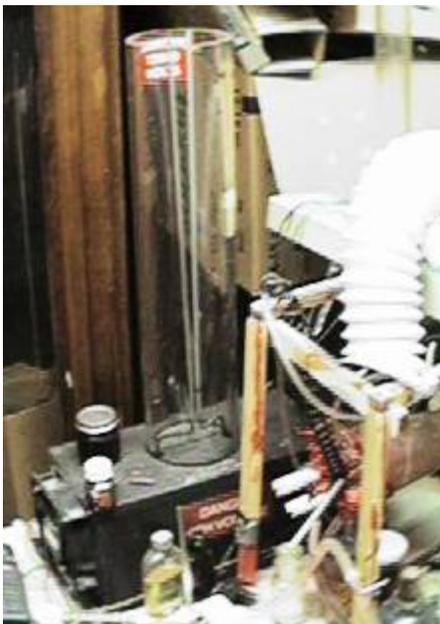
A 7,500 volt spark climbs an 18" Jacob's ladder making a nice "buzz.... pop!" sound. It's powered by a neon sign transformer bought at a surplus store for \$35. This is a *lethal* voltage/amperage. The spark will set a piece of paper on fire. The visitors are kept away from the table (for obvious reasons) by a metal mesh stapled to a wooden frame screwed into the doorway. The Jacob's ladder has a cooling fan on the side.
