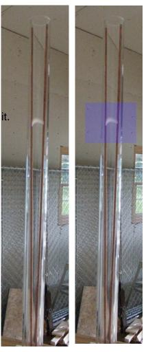
Here is the working ladder. Both pictures are the same but the one on the right has the arc highlighted in a blue shade. Even though the ladder is encased some what it doesn't mean it is safe. You should not leave this running unattended or leave it in place where some unsuspecting person might get their hands on
