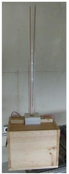
When the arc would stall it would cause the copper plating to scare and after awhile the arc would not travel very well for some reason. The pure copper rods worked best in my opinion.
