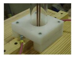
The white plastic stuff is Tivar 1000. We use it at work and I was going to try to put the copper rods in that but at times this stuff would catch fire and start to melt when the arc started so I dropped that idea and went with the 2x4. Although it worked great to secure the acrylic tube in place. I'm sure you could use any kind of lumber if you decided to build one like this
