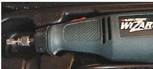
The tool of choice for me on this project was a Black & Decker Wizard. Any Dremel type tool will work, but you definitely need some such tool as you'll be doing a lot of grinding away of the skull's interior plastic to make room for the gear assemblies. I used the Dremel bit that is shaped like a pencil eraser with deep diagonal ridges, cut through
