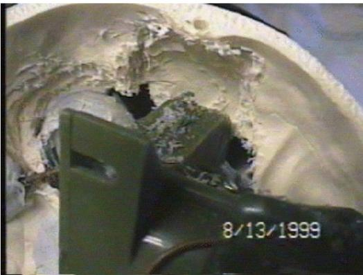
To mount the motor/eye assembly, grab your dremel and prepare to grind! You want the front end of the green plastic motor housing to be installed right behind the bridge of the nose of the skull. You'll probably find as you eyeball the placement (pardon the pun) that such a placement will keep the eyes too far back. Grab that dremel and start grinding away the plastic behind the bridge of the nose. You want to keep grinding away until the whole assembly
